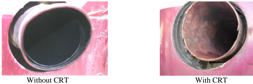
Fig. 3: Bus tailpipe view with and w/o the CRT.
