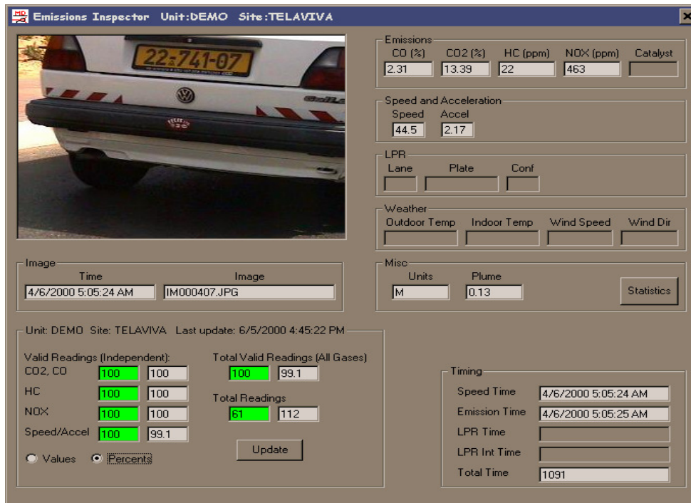
Figure 3. Output of the computer display after measurement (Israel, April 2000)
